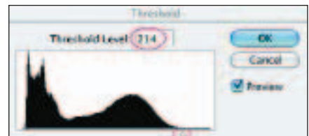
FIGURES 3-9A AND B. THRESHOLD. The dialog box indicates that the Threshold Level for the highlights in the image is 214. This corresponds to the image highlights visualized as white pixels in figure 3-5.
